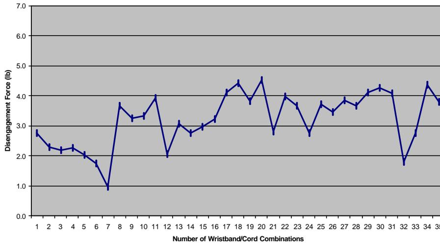
Figure 2. Breakaway Force Data for Wristbands with Machined Snaps
