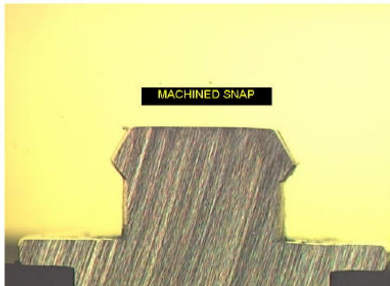
Figure 4. Cross Section of a Machined Snap
