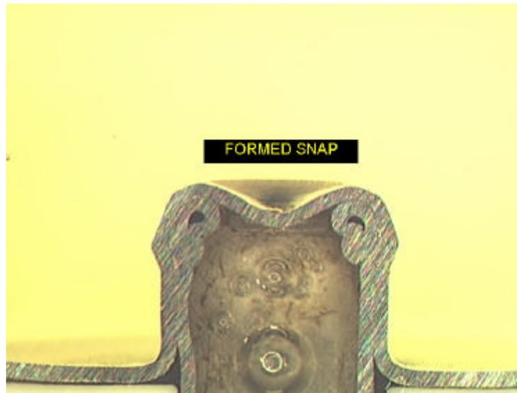
Figure 3. Cross Section of a Formed Snap
